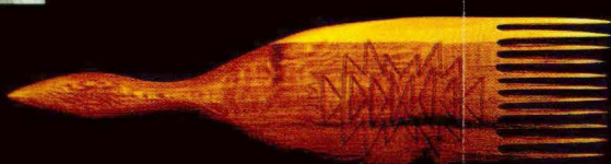
Weaving forks, like this one, are used to pack down the weave as a weaver works.
