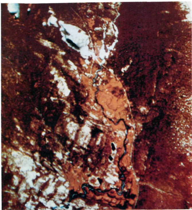
Fig. A. Color infrared rendition of aircraft scanner data used to produce thematic landcover classes. (Resolution = fifteen meters).
