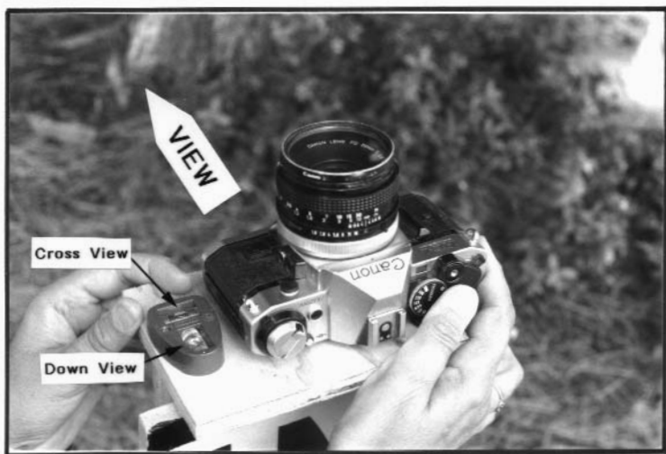
Figure 27—System to photograph tree canopy cover. The photo point meter board will be crosswise of the view. Place the camera level board on top of the meter board and the camera on the level board. First, center the cross-view level by moving the meter board sideways. Then tilt the camera level board so that the down-the-view level is centered, move your head out of the camera view, and photograph.
