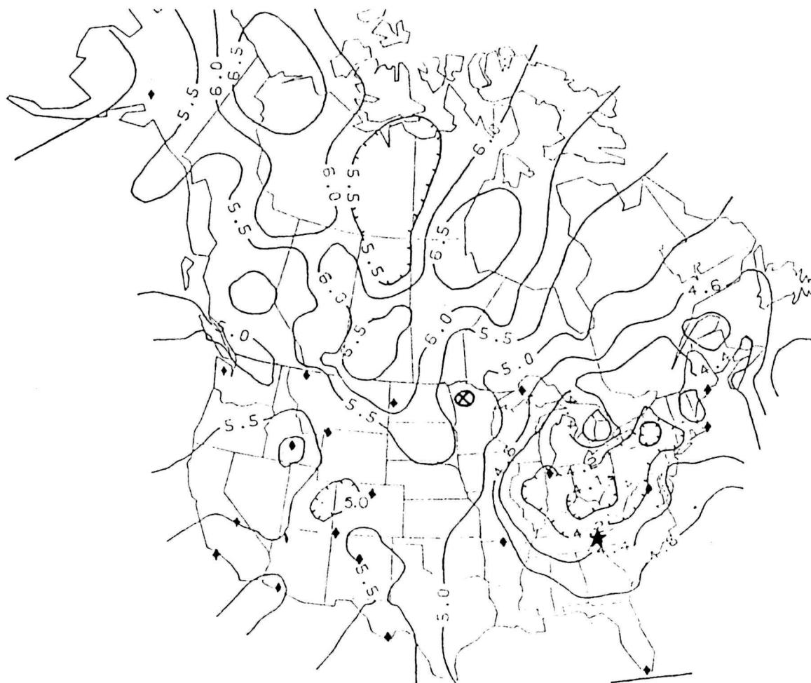
Figure 3. Isopleth of the United States showing the distribution in rainfall pH for the year 1981. Diamonds represent NPS/NADP sites. (NADP, 1982)
