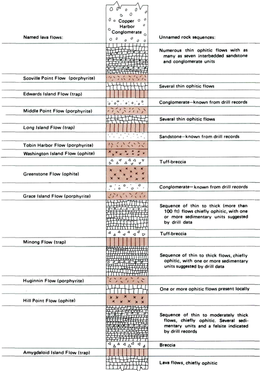
PORTAGE LAKE VOLCANICS—schematic columnar section on Isle Royale. Not drawn to scale. (Fig. 17)
