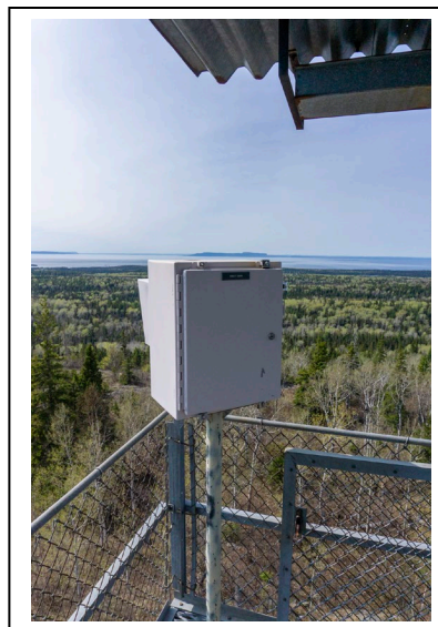
Figure 23: Ojibway Fire Tower visibility monitoring camera on northwest corner of balcony, looking northwest. Photo by Natalie Young, 2019.
