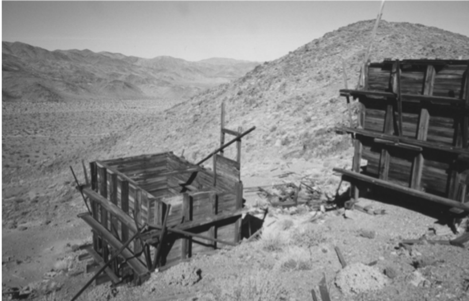
Figure 2: Tipples (ore bins) at the Silver Bell Mine site, Joshua Tree National Park, Photo by D. D. Trent, 2001.
