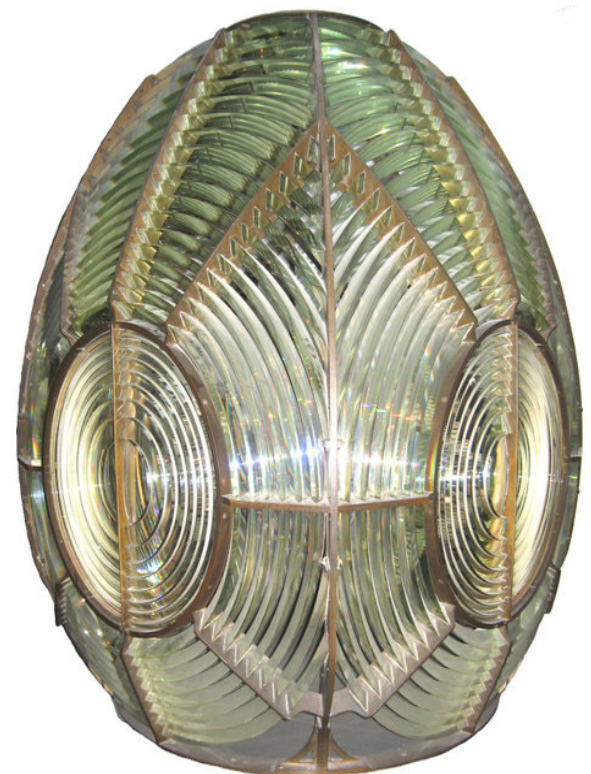
The second-order Fresnel Lens is six feet in diameter.
