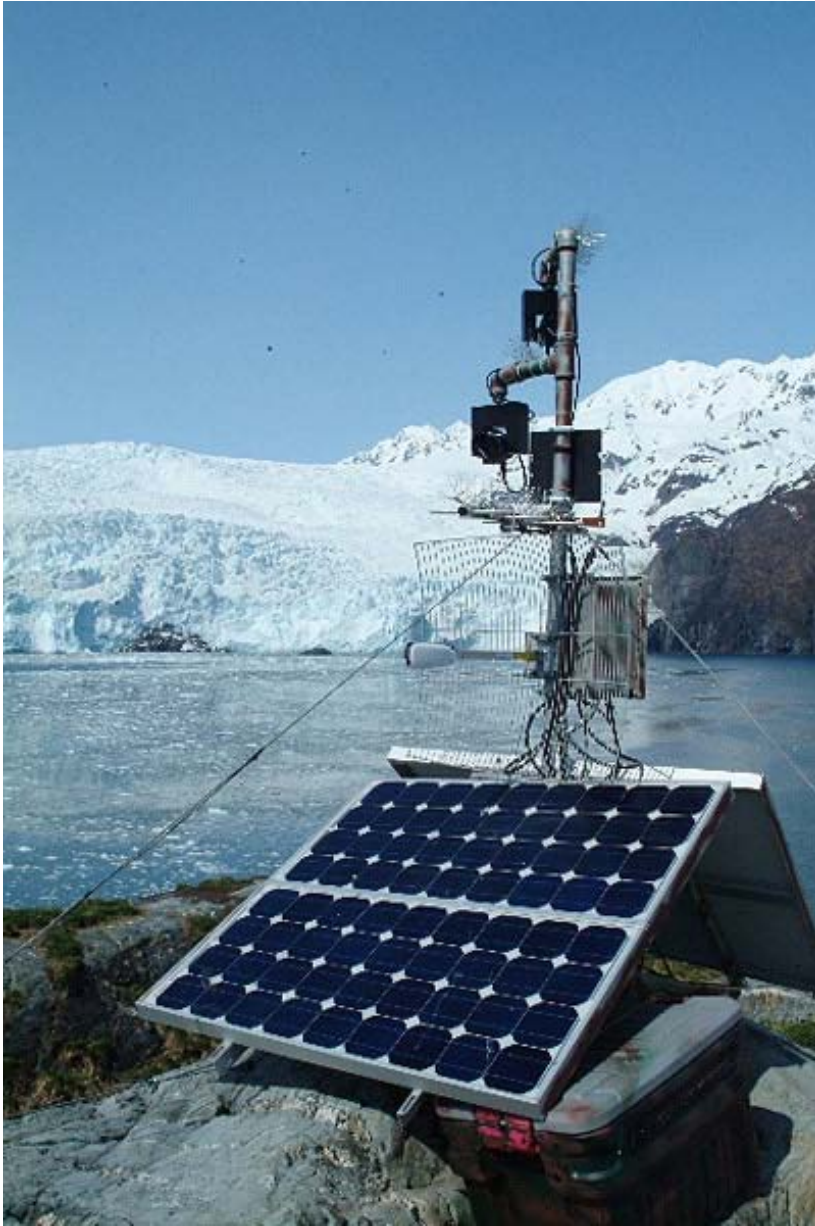
Figure 20. One of the remote cameras located on Squab Island near the face of Aialik Glacier relays live video of harbor seals adjacent to the glacier. http://www.oceanalaska.org/research/sealrvm-images.htm
