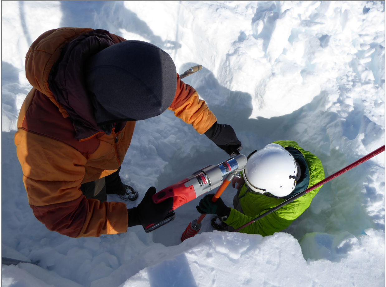
Figure 5. Lowering the Kovacs corer into the hole to sample below the two-meter-deep floor of the snow pit. NPS / D. KURTZ
