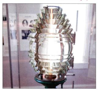
A Fresnel Lens sent out light signals from the Eagle Harbor Lighthouse tower to passing ships for much of the Lighthouse's history. The Fresnel Lens lit the way with a variety of illuminants, including whale oil, lard oil, kerosene and electricity, until it was replaced in the 1960s with an Aviation Beacon with red and white lamps. Currently, a Marine Rotating Beacon, is beaming out signals from the tower. It is fully automated and is maintained by the U.S. Coast Guard.
