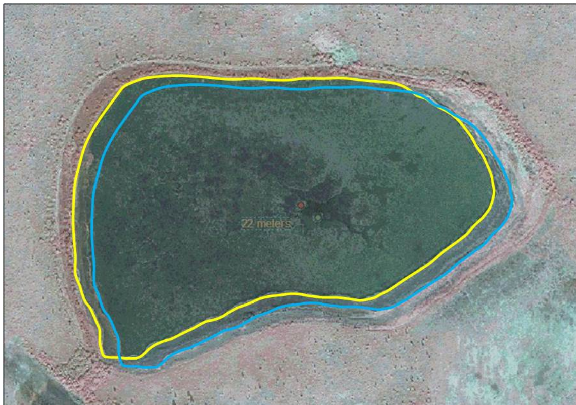
Figure 2. Shift between SPOT 5 DEM spatial corrections (highlighted in blue) versus original IKONOS DEM spatial corrections (highlighted in yellow).
