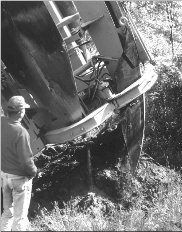
A tree spade can be used to remove stumps in locations where the use of larger equipment will not damage resources.
