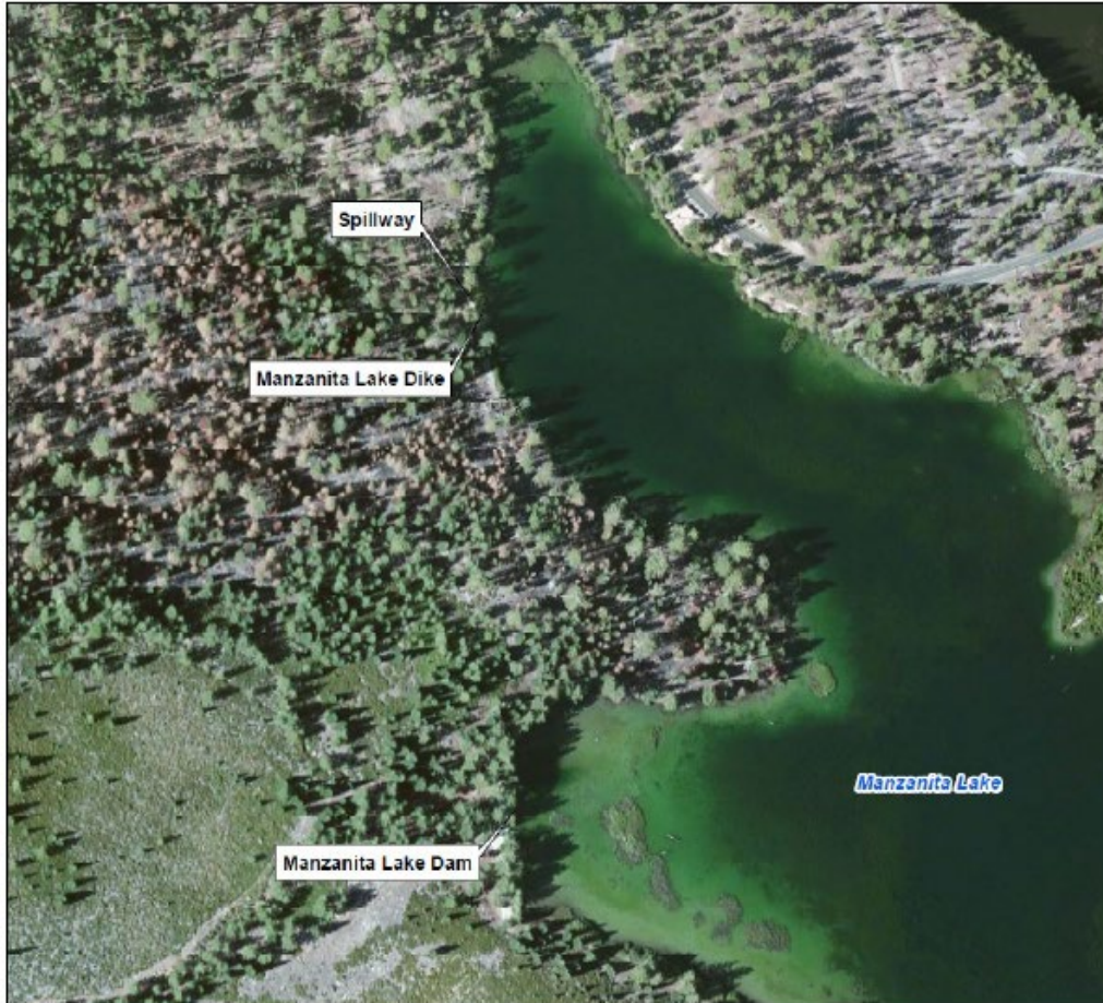
FIGURE 19. ARIEL VIEW OF THE DAM, DIKE, AND SPILLWAY FOR TERMINOLOGY USED IN THIS PLAN (NPS 2021A, FIGURE 2)
