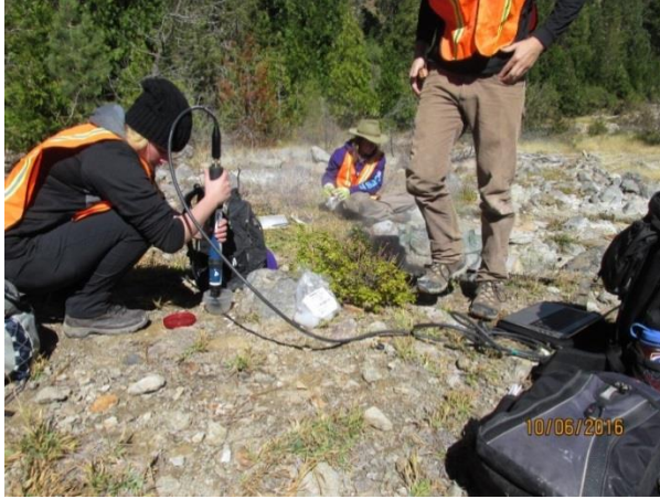
Figure 8: Undergraduate assistant Ashley Stewart analyzing a water sample with the Hydrolab Sonde.
