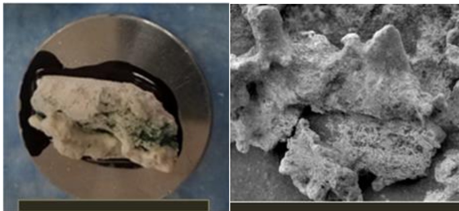
Figure 33: Side-by-side comparison of amorphous silica precipitate sample L-17-DK-04 Coating (left) from Devil's Kitchen and the Elizabeth Mahon Target from Home Plate (right). Both samples have a similar lobate morphology with regions of a smooth texture and regions of a more porous texture. The black scale bars at the bottoms of both images is ~2.5 cm.
