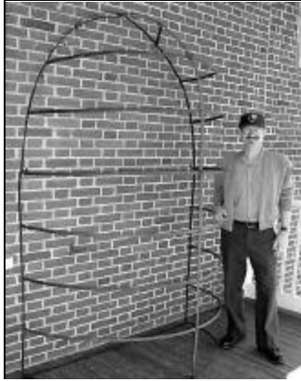
Fig. 9. Reproduction of a section of the collapsible iron boat frame fabricated at the Harper's Ferry Armory. Source: National Park Service, October 2002.
