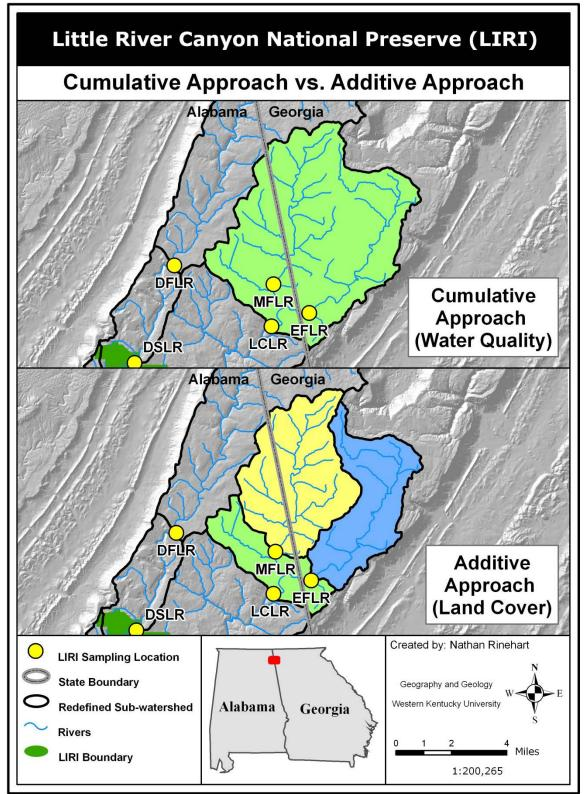
**Figure 12.** Cumulative approach vs. additive approach for defining sub-watersheds at Little River Canyon National Preserve. DFLR – DeSoto Falls, MFLR – Middle Fork Little River, EFLR – East Fork Little River, LCLR – Lookout Mountain Camp, DSLR – DeSoto State Park. Source: Author, (USGS 2007a).
