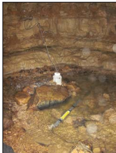
Figure 4: Photograph showing the pool at the bottom of Annette's Dome and the beginning of Shaler's Brook. Also pictured is the YSI datasonde with the first flush sampler.
