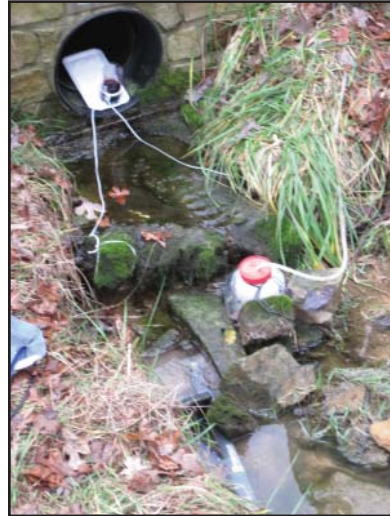
Figure 3: Photograph showing the dye and salt release mechanism. Also shown in the picture are the first flush sampler and the YSI datasonde.
