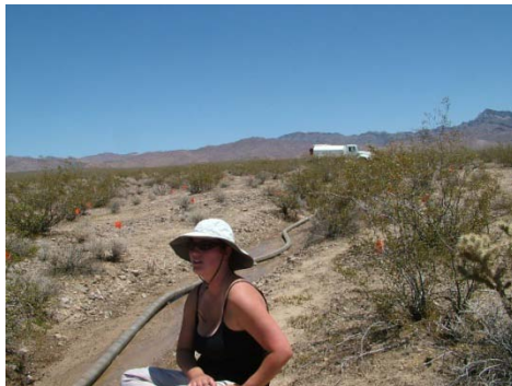
A water truck and perforated hose were used to simulate runoff in a small alluvial channel.
