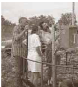
Miguel Flores (right) demonstrates how to change a particle filter at an air sampling site east of San Antonio, Texas.
