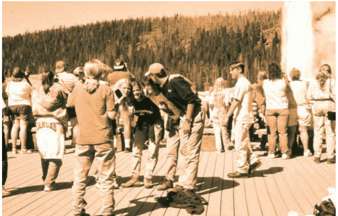
The massive viewing platform at Old Faithful Geyser in Yellowstone is constructed of recycled-content plastic, demonstrating to thousands of tourists daily the practicality of this tough and sensible wood alternative. Unilever Home and Personal Care—USA, in conjunction with a cost-share agreement with the park, obtained the plastic lumber, valued at over $300,000, which was produced from the equivalent of more than 4 million plastic milk jugs.
