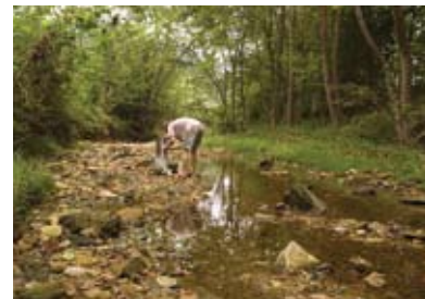
Researcher Jason Robinson sets up an ultraviolet light trap along South Knob Creek at Abraham Lincoln Birthplace National Historic Site in Kentucky. A photocell turns the light on when the sun sets and off when the sun rises, allowing unattended operation.
