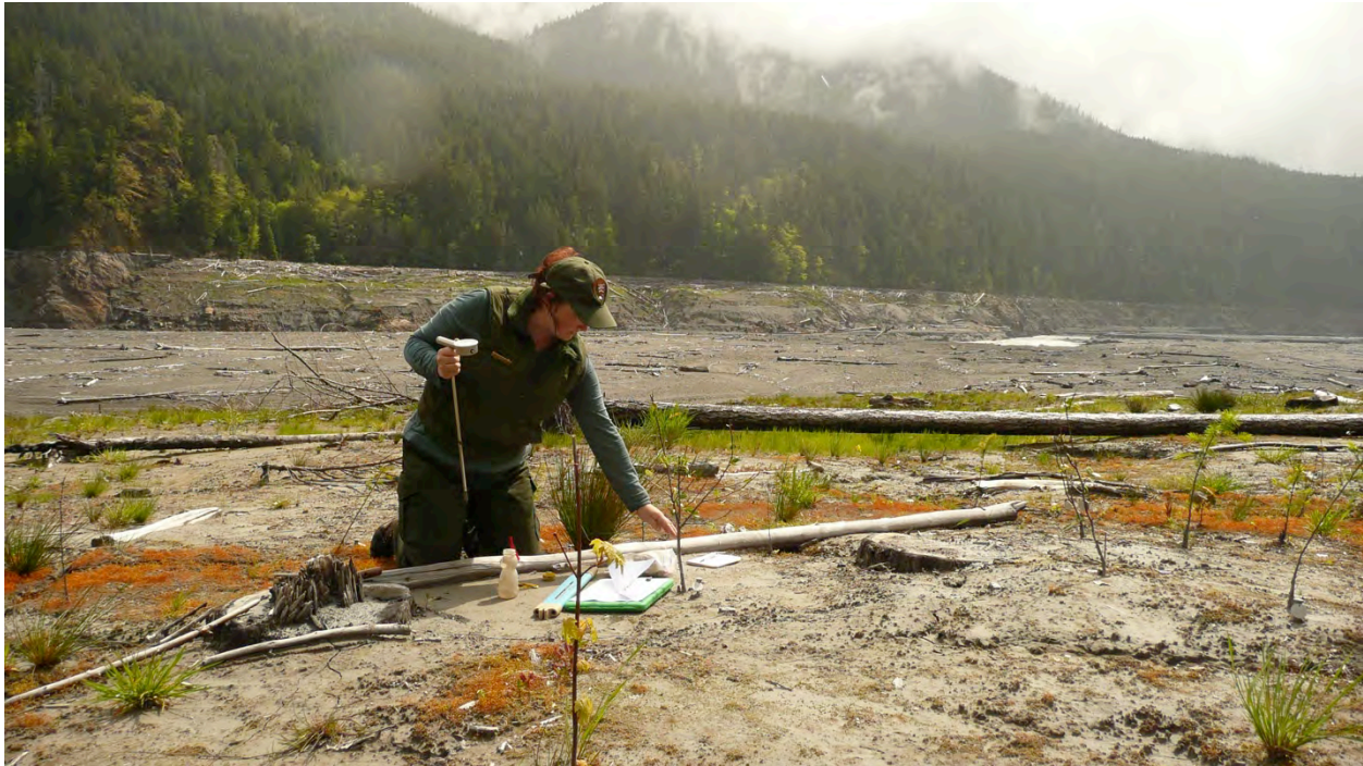
Figure 25. Marisa Whisman taking tensiometer measurements in the sediments of the former Lake Mills.
