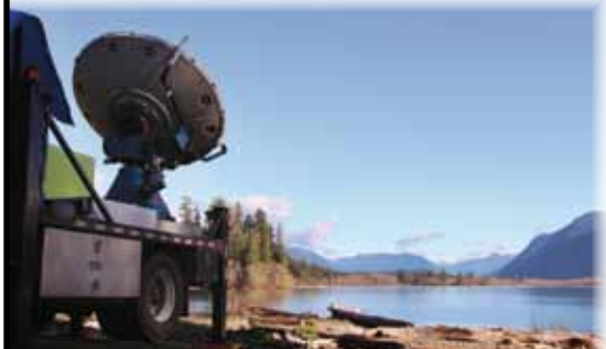
Mobile Doppler radar collects data at Lake Quinault.
