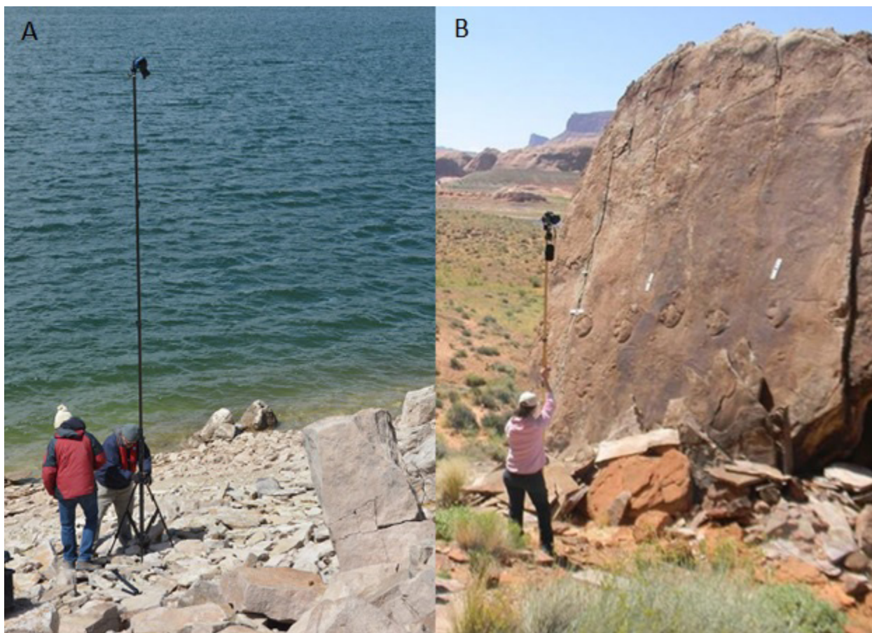
FIG. 1. (A) Using the camera mast to photograph from an elevated position to document areas on the ground. With unmanned aerial systems restricted in National Park Service areas, this method allows for systematic low-altitude aerial imagery. (B) Using a camera mast to capture imagery nadir to a vertically oriented surface to ensure photograph overlap and proper spacing for a 3D model. Note the scale bars (white rectangular objects) on the surface of the track block.
