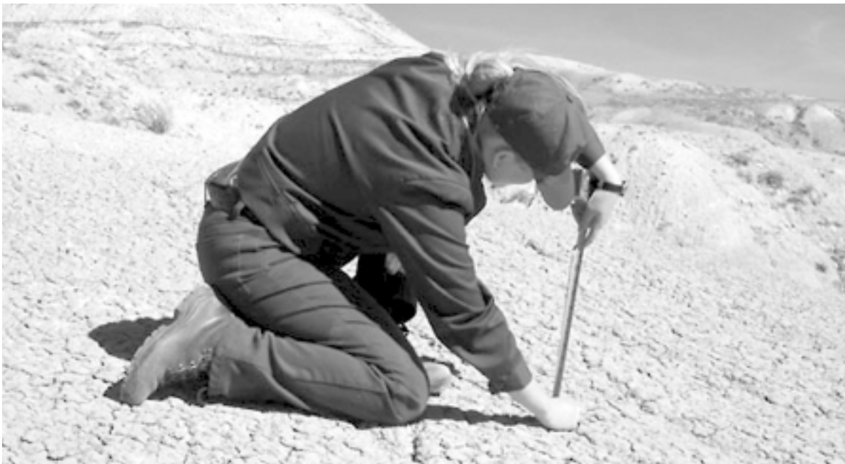
Figure 2. A primary factor in fossil stabilization, erosion is monitored closely by park staff at Fossil Butte National Monument, Wyoming. Changes in measurements between the substrate and the top of a reference stake (not visible) are recorded along with local temperatures, precipitation, wind speed, and other factors that affect erosion. Together, the data help the park anticipate management action necessary to preserve park fossils.
