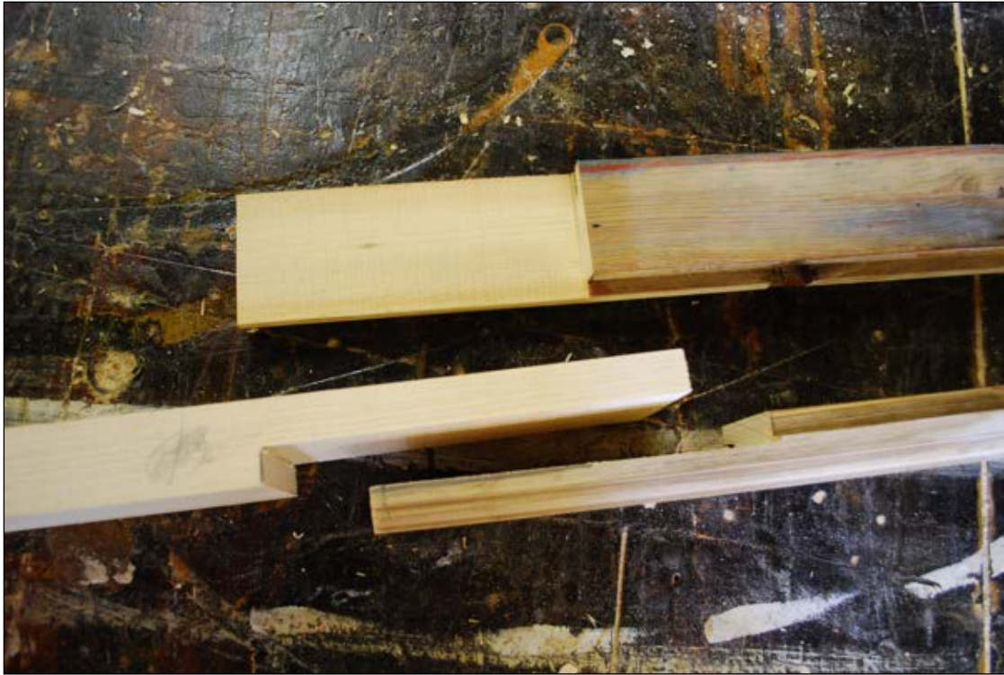
Figure 4. Half-lap joint prior to gluing.
