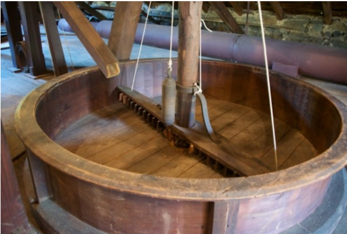
The hopper boy machine. (photo courtesy of William Mills)
