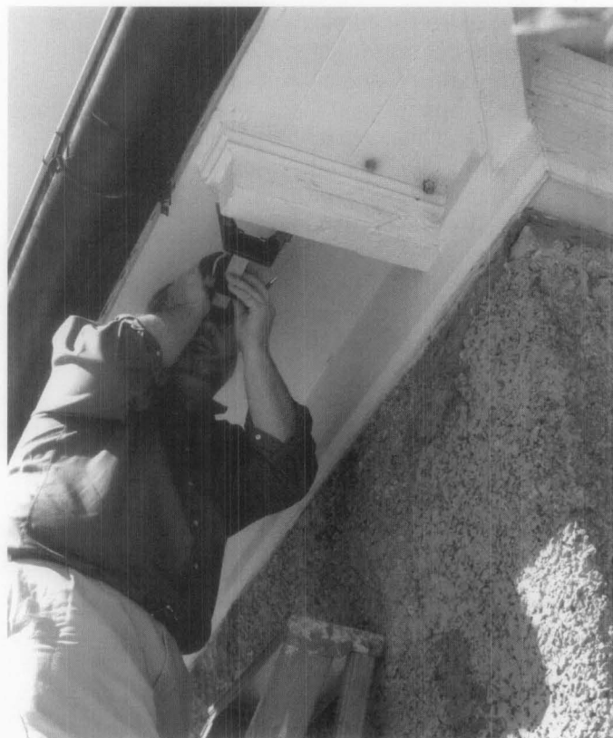
Figure 13. Paint studies may not only help establish the chronology of paints and paint colors used on a building but also may aid in the dating of existing architectural features. Examination of the paint layers on these modillions utilizing a hand-held microscope enabled an investigating team to confirm in the field which modillions were original and which were later replacements. Photo: Charles Fisher, National Park Service.
