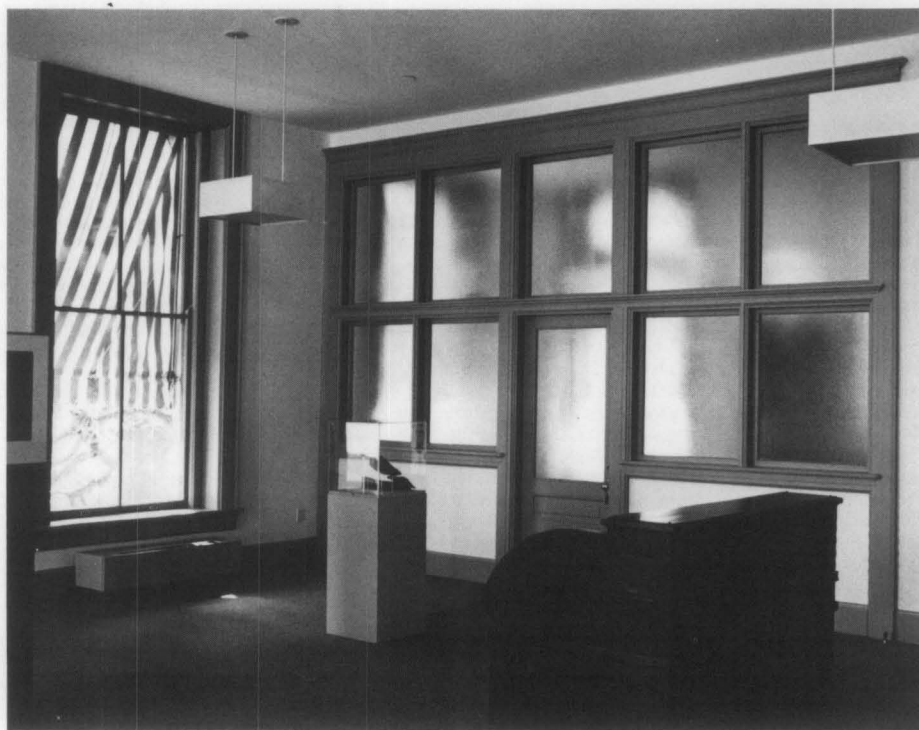
Figure 3. By reducing the glare and solar gain, the awnings have eliminated the need to purchase and maintain interior shades and draperies in various offices. Photo: Courtesy, Florida Bureau of Historic Preservation.
