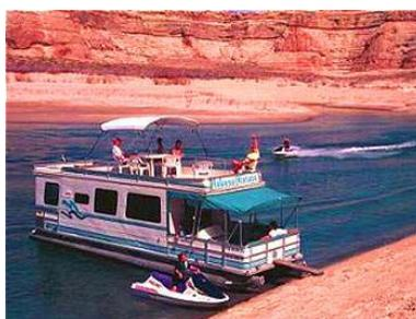
Gasoline-powered engines on houseboats, including the houseboat's onboard generator, produce carbon monoxide, a colorless and odorless gas that can poison or kill someone who breathes in too much of it. Carbon monoxide tends to build up above the water near the water platform. The amount of carbon monoxide that can build up in the air space beneath the stern deck on houseboats can be deadly within seconds to minutes and can also reach life-threatening concentrations on and near the swim deck.
