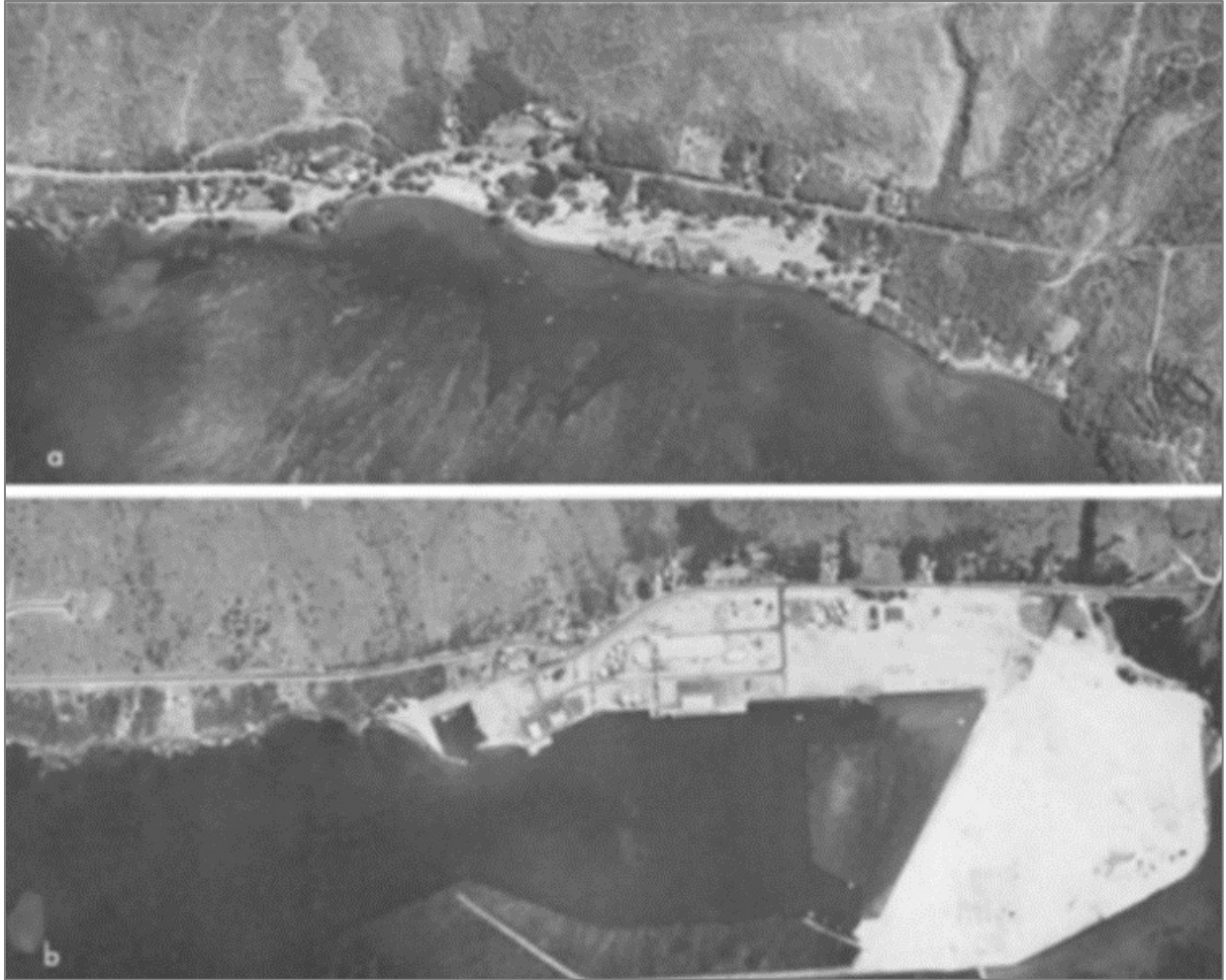
Figure 16. Shoreline before (top) and after (bottom) harbor construction. Pu'ukoholā Heiau is visible in the lower right corner of the upper image but is out of view in the lower image. The channel of Makeāhua stream enters the upper image just below the upper right corner but is out of view in the lower image. The upper image shows the position of Makeāhua stream prior to being rerouted towards the south (to the right in this image; MKSWCD 2005). Additional images may be viewed at http://kawaihaereef.org/archives
