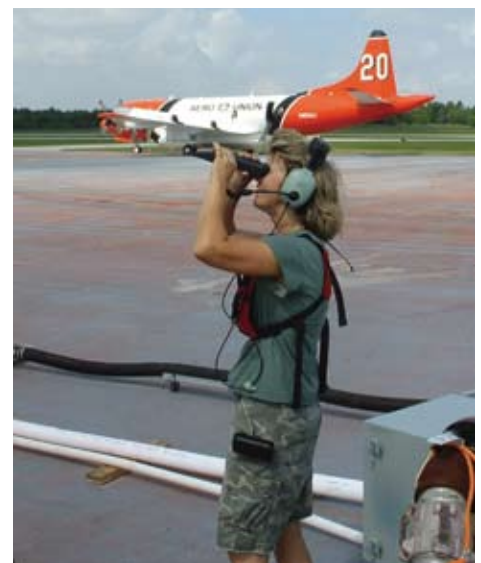
Maintenance Worker Gina Smith uses a refractometer to measure the salt content of fire retardant in Ocala, FL.
