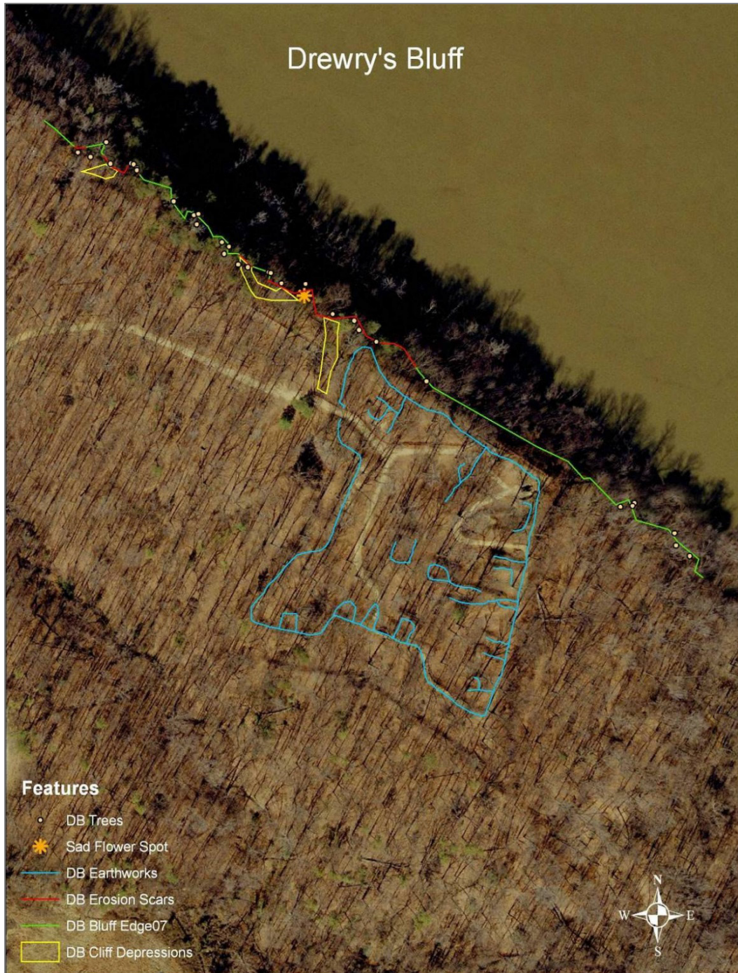
Figure 21. Aerial photograph of Drewry's Bluff with GPS-located features. White dots represent trees at the bluff crest, red lines are erosion scars, green lines are the bluff crest, yellow areas are cliff depressions, and blue lines outline the earthworks associated with the cultural resources at the site. The "Sad Flower Spot" refers to an unofficial memorial site (with flowers) that had been established near the bluff edge around the time of the map's creation. A correlation seems to exist between erosion scars and depressions (e.g., trenches funneling water toward the bluff), while more stable bluff segments are occupied by trees. Graphic by K. Allen and A. Trivizas (Richmond National Battlefield Park) presented as Figure 1 in Gerstel 2008.
