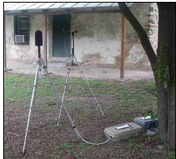
Photo 24. Sound monitoring equipment at Tufa House (NPS photo).
