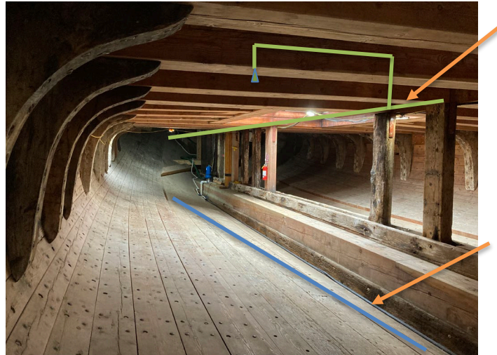
Photo 9: If the entire hold, in its present arrangement, of the ship is water mist protected then a main tube will run along the approximate center and 12 mm branch lines will be routed from the main to the nozzles. If the deck houses alone are protected and a single cylinder set is located on the hold deck, the 25 mm main tube will follow a similar route, or may be integrated along the keelson and run vertical into the deck houses.
