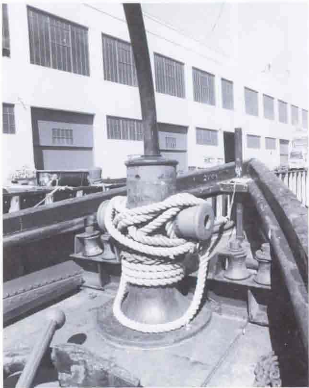
Fig. 24. Kingpost bitt on foredeck, one of several original custom-made items HERCULES is fitted with. Roller-chocks to port and starboard of the bitt are a later addition.
