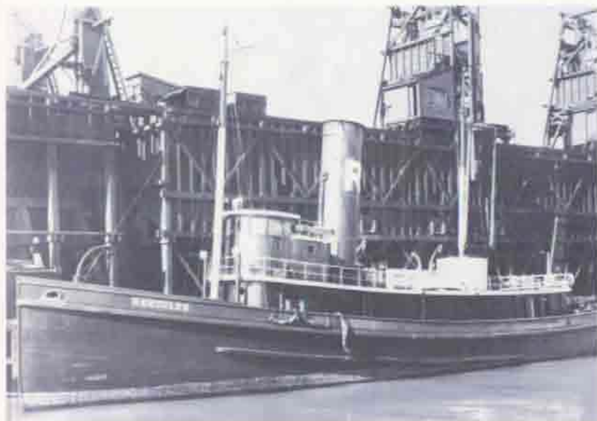
Fig. 5. HERCULES in the colors of the Rolph Coal and Navigation Company; black stack with large white "R." Note wireless stacks at mainmast, and antenna wires between masts.
