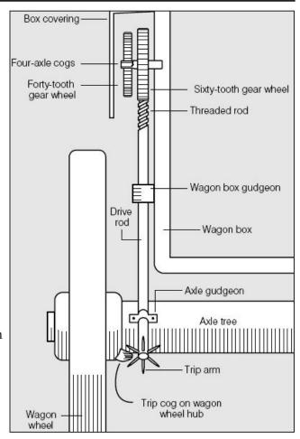
The axle of the 60-tooth gear wheel has 4 cogs cut into it. These work on a second gear wheel of 40 teeth. With every rotation of the 60-tooth wheel, 4 teeth of the 40 tooth wheel will be drawn by, each representing a quarter of a mile.
