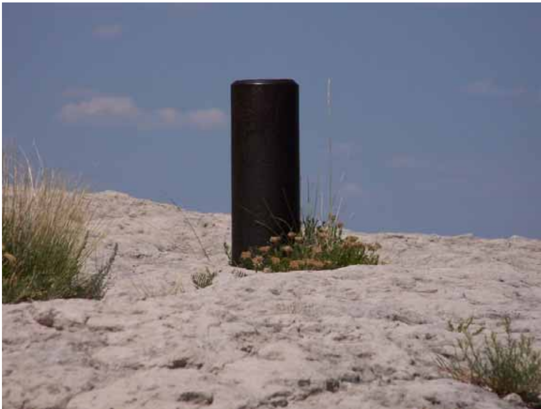
Figure 8. Erosion on Scotts Bluff. Erosion has exposed about 0.3 m (1 ft) of this metal survey post, which was level with the surface when installed on the summit of Scotts Bluff in 1933. The survey marker shows the elevation of Scotts Bluff in 1933 to be 1,417 m (4,649 ft) above sea level. Photograph by John Graham (Colorado State University), July 7, 2007.
