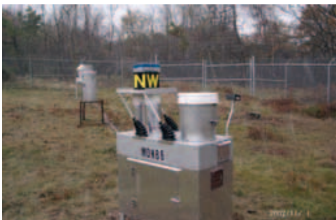
Figure 2. Views of MDN sites VA-08, Culpeper (top), and VA-28, Shenandoah National Park-Big Meadows (bottom). Each station consists of a recording rain gauge (cylinders) and a precipitation collector (boxes). Mercury sample is collected through a glass funnel exposed when a moisture sensor activates the lid covering the sample chimneys at the left side of the collector. Top photograph by Allan Kolker, USGS; bottom photograph from National Atmospheric Deposition Program ( http://nadp.sws.uiuc.edu/sites/siteinfo.asp?net=MDN&id=VA28 ).
