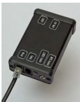
Figure 4.8: Data/power connection between interface box and LD831
