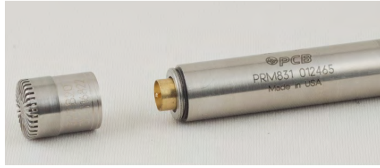
(a) Detaching the microphone capsule
