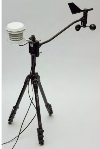
Figure 3.5: Relative humidity / temperature probe mounted on tripod with an anemometer
