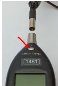
Figure 4.6: Audio connection between interface box and LD831
