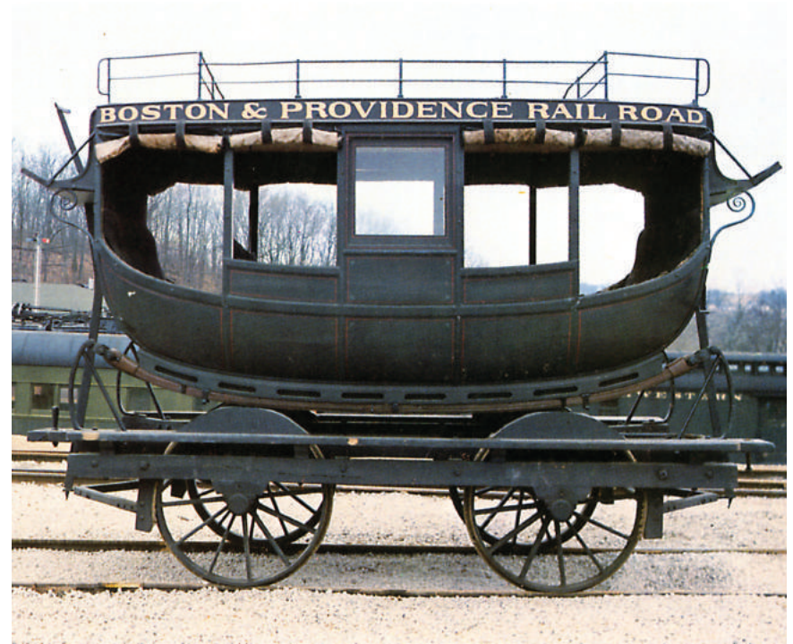
This stagecoach-style passenger car was built between 1834 and 1836 by John Lightner for the Boston & Providence Railroad and is now displayed in the National Museum of Transportation in St. Louis. It is the oldest surviving original railroad passenger car in North America and may have been similar in design to the passenger cars used on the Tuscumbia, Courtland & Decatur Railroad during the Cherokee removal. Courtesy of The National Museum of Transportation, St. Louis, Missouri.
