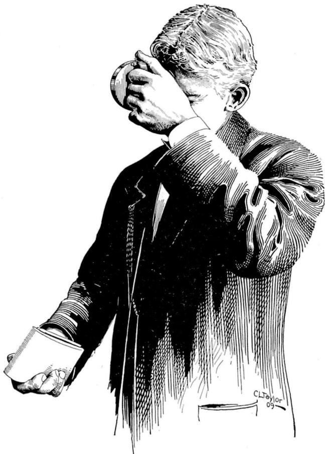
FIG. 10.—Method of sighting with standard hypsometer.
