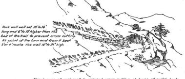
Showing use of rock wall to prevent cross cutting at turns of switch backs. Use only where rock of substantial sizes are handy.
