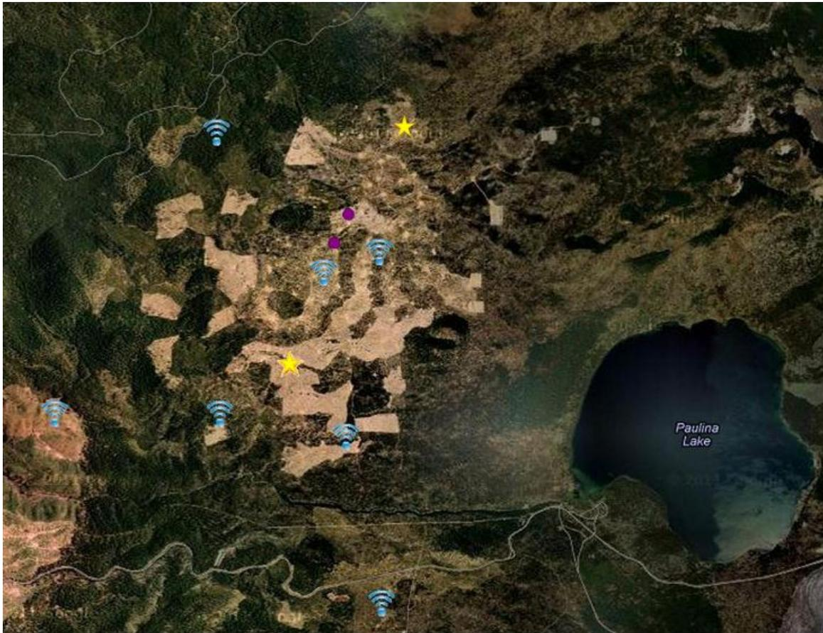
*Figure 13: Earthquake locations from Ernie Major (Lawrence Berkeley National Laboratory) data. Purple dots are the earthquake locations. Yellow stars identify 55-29 (south) and 46-16 (north) well locations.*
