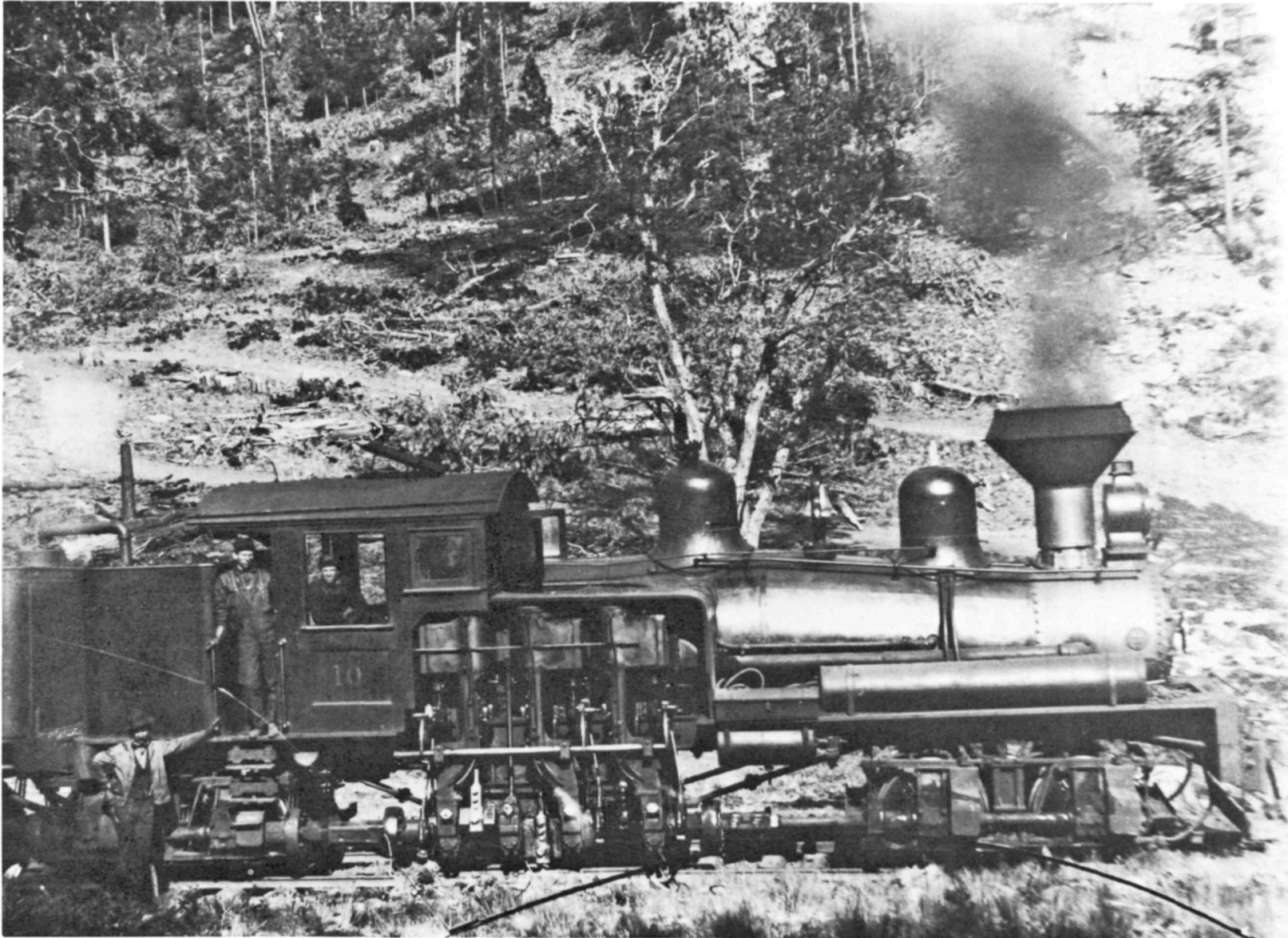
Figure 12. Zuni Mountain Railway Shay locomotive Number 10. This view clearly shows the drive system of the Shay, with the main shaft extending forward and aft from the three cylinder main engine of the locomotive. Between the engine and the trucks were universal and slip joints to allow the locomotive to round curves, and the shaft drove each axle through bevel gears. Although mechanically inefficient and noisy, the Shay was a very practical and popular logging locomotive. Cibola National Forest collection.
