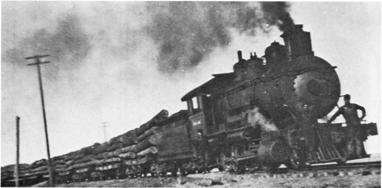
Figure 13. Zuni Mountain Railway's 133 ton 2-8-0 locomotive Number 12. John P. Bigley collection.
