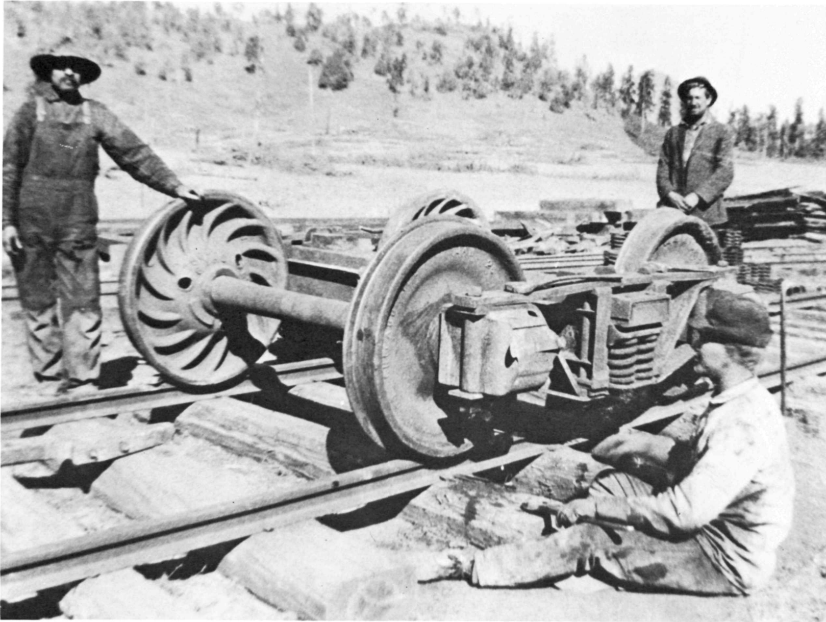
Figure 61. Three "car tonks" -- railway mechanics -- working on an arch-bar freight car truck at Kettner, circa 1908. This type of truck, bolted together of individual parts, was soon superseded by massive cast trucks. John Bigley collection.
