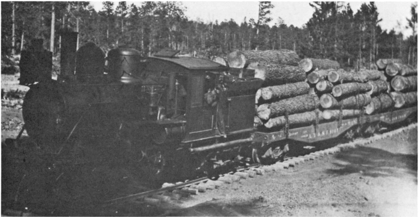
Figure 57. The Climax gear-drive locomotive, Zuni Mountain Railway Number 8, heads for camp with loads of logs. Cibola National Forest collection.
