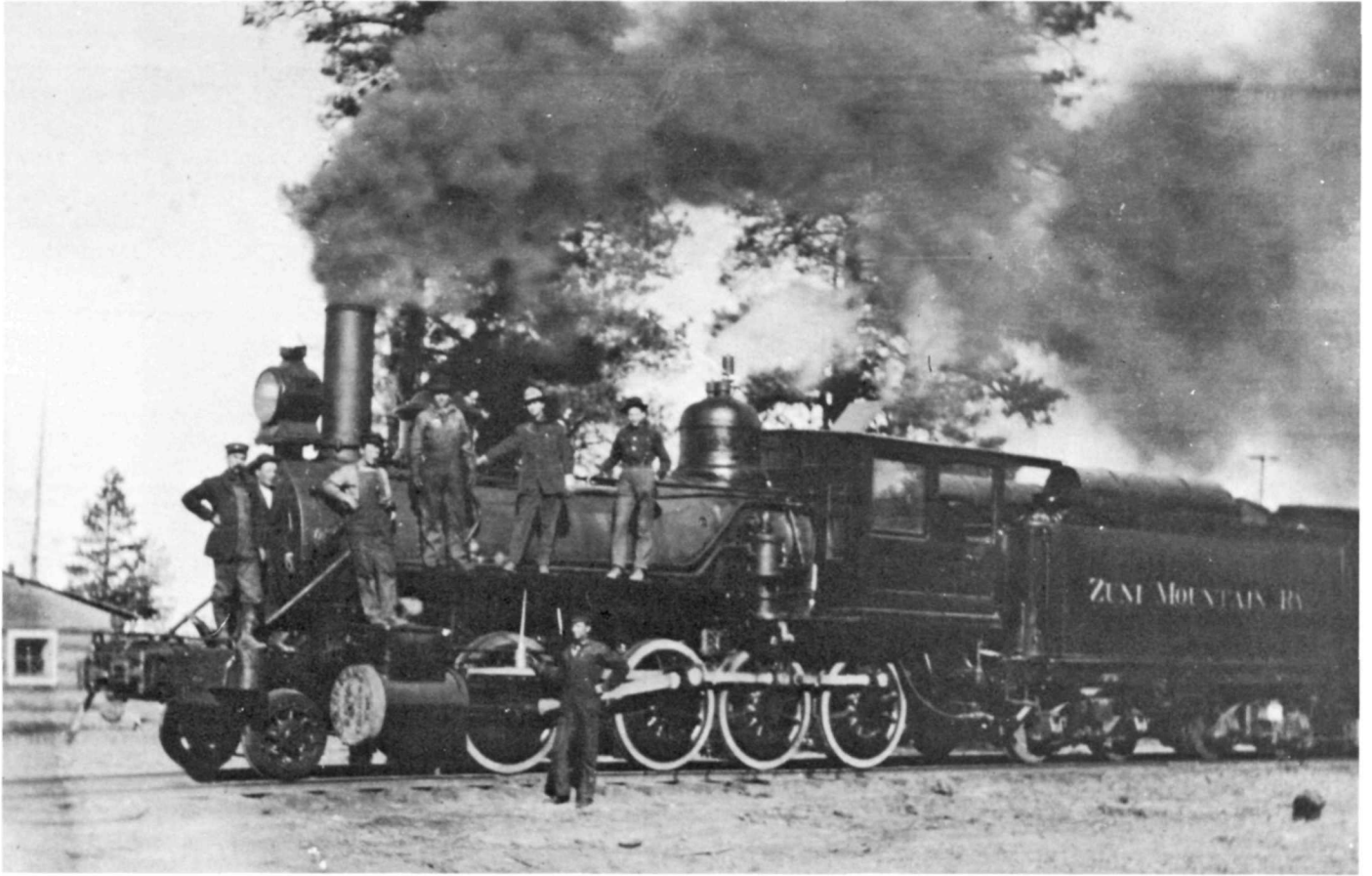
Figure 28. Old "mainline" locomotive Number 6 of the Zuni Mountain Railway. This ancient eight-driven freight locomotive was used to haul log trains from the woods camps to the connection with the Santa Fe Railway at Thoreau. Cibola National Forest collection.
