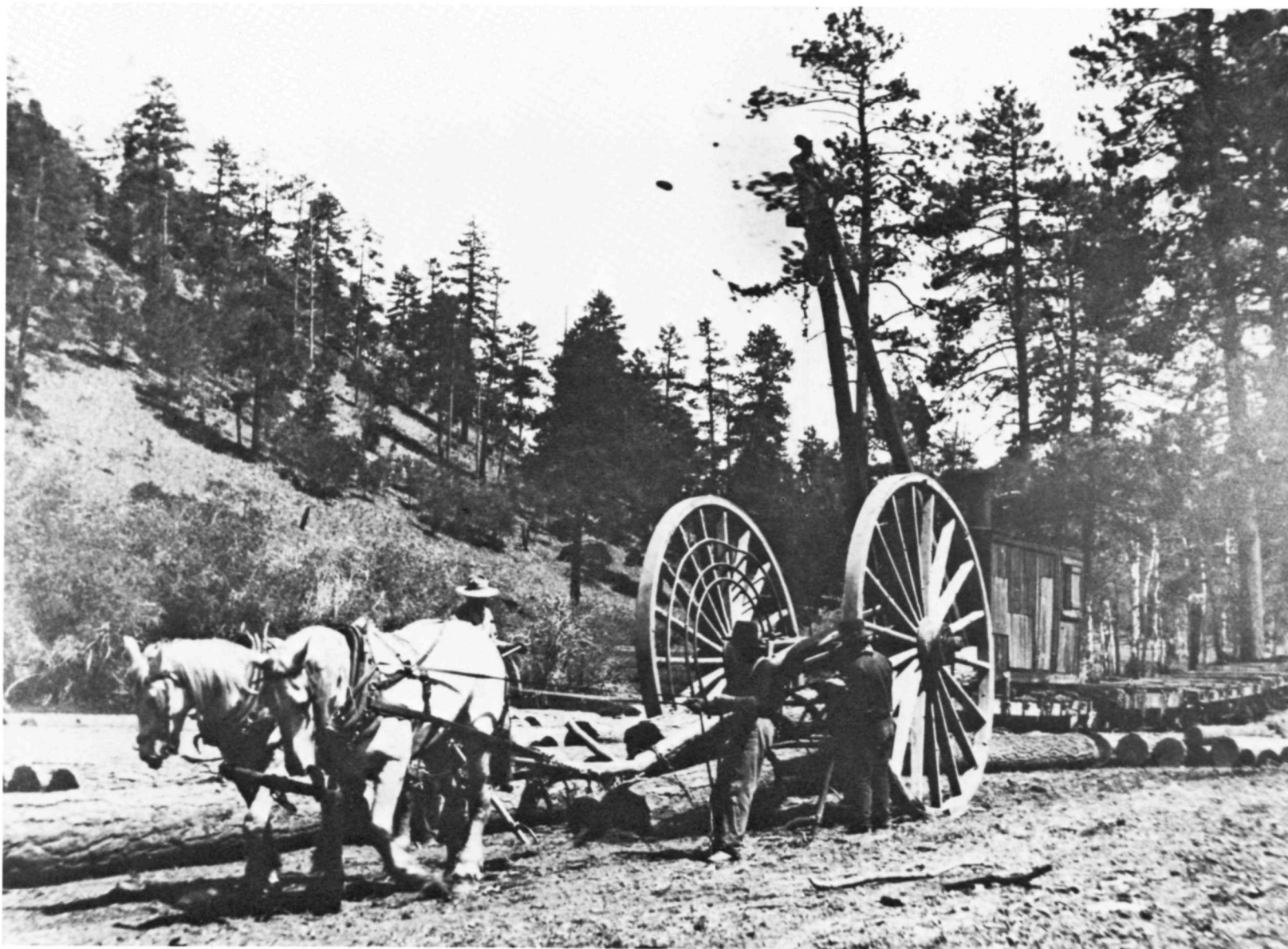
Figure 22. A two-horse team with big wheels ready to drop its load of logs at a railroad landing. One of the American Lumber Company loaders and a string of cars waits in the background ready to go to work.
