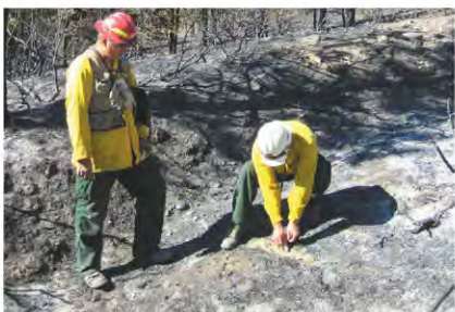
SOIL PERMEABILITY TESTING IN A BURNED AREA
