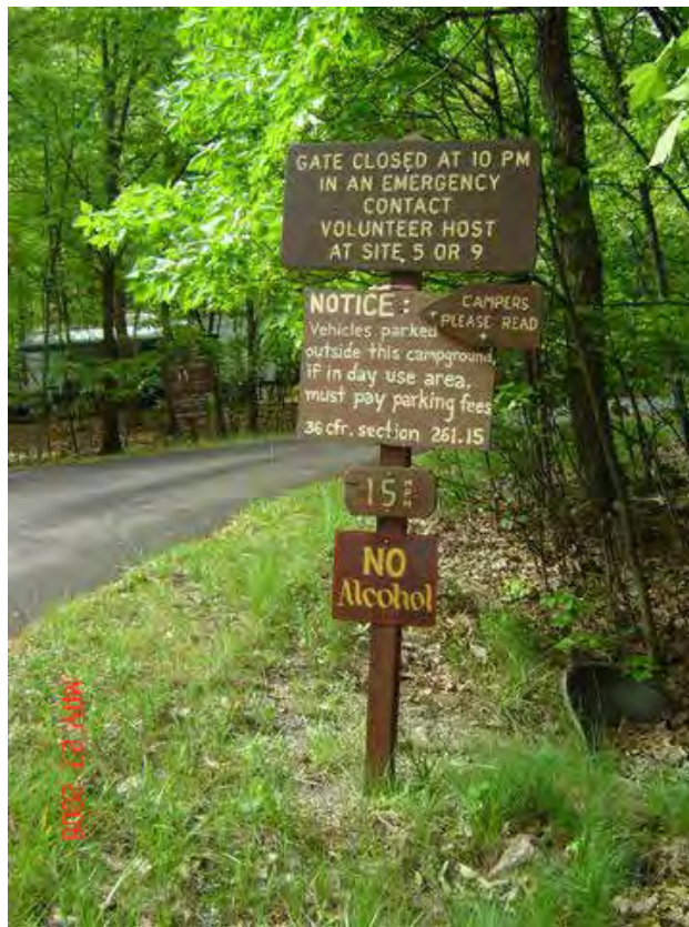
Figure 10B-5—Example of homemade VIS. It appears that this sign is to be read from a moving vehicle; this is not appropriate for VIS. Do not post VIS information next to a road. On these signs, there is too much text, it is too small, and it cannot be read from a moving vehicle. Sign placement could cause safety problems; drivers must stop to read the information. Information needed to be read from a moving vehicle, such as the speed limit, shall meet all of the requirements and standards in Chapter 3—Traffic Control Devices.
