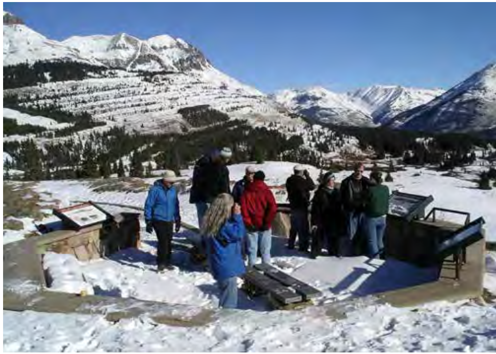
Figure 10A-12—This panorama interpretive plaza is well defined, has low profile signs so one can see what is being interpreted, and a bench. The base is native stone. Molas Pass, San Juan Scenic Skyway, San Juan National Forest. Rocky Mountain BEIG Province.
