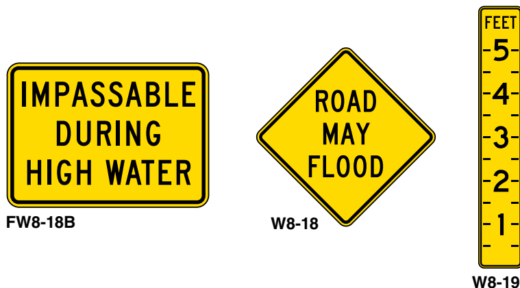
Figure 7-17—Flood warning signs for roads.
