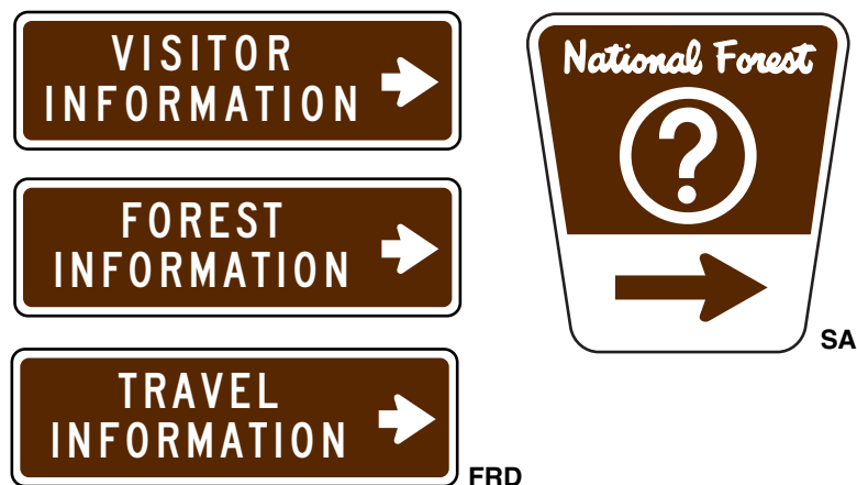
Figure 6-12—Advance guide signs for travel management information.
