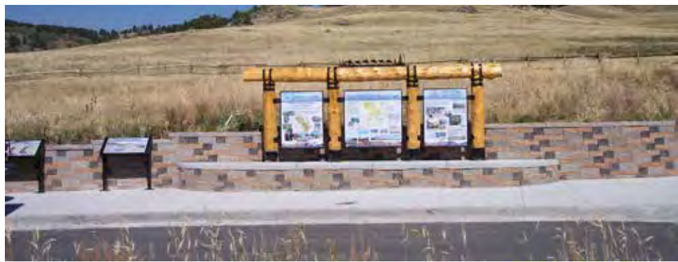
Figure 10A-14—Signs are legible from a vehicle in the pullout; one can park and read the low-profile signs as well. Hospital Hill, Cloud Peak Skyway, Big Horn National Forest. Rocky Mountain BEIG Province.
