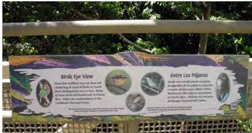
Figure 10A-17—Bilingual sign made of a plastic embedment that has been in the tropical climate since 2004 (for 6 years). El Yunque National Forest. Southeast Coastal BEIG Province.
