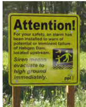
Figure 7-16—Example of a sign posted below a dam.
