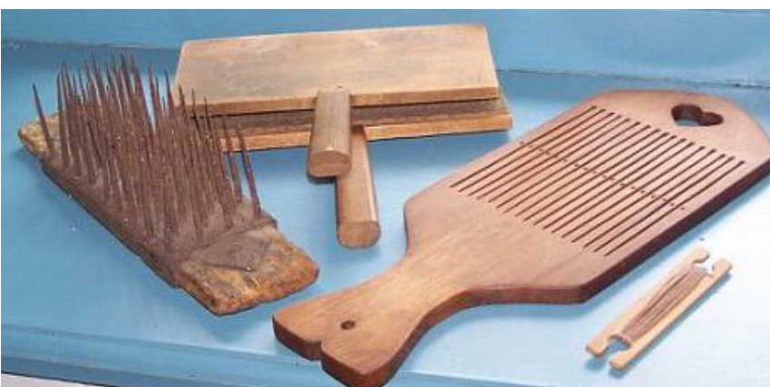
VAFO 2560 Hatchel; VAFO 2658 Carding Combs; VAFO 3319 Loom
