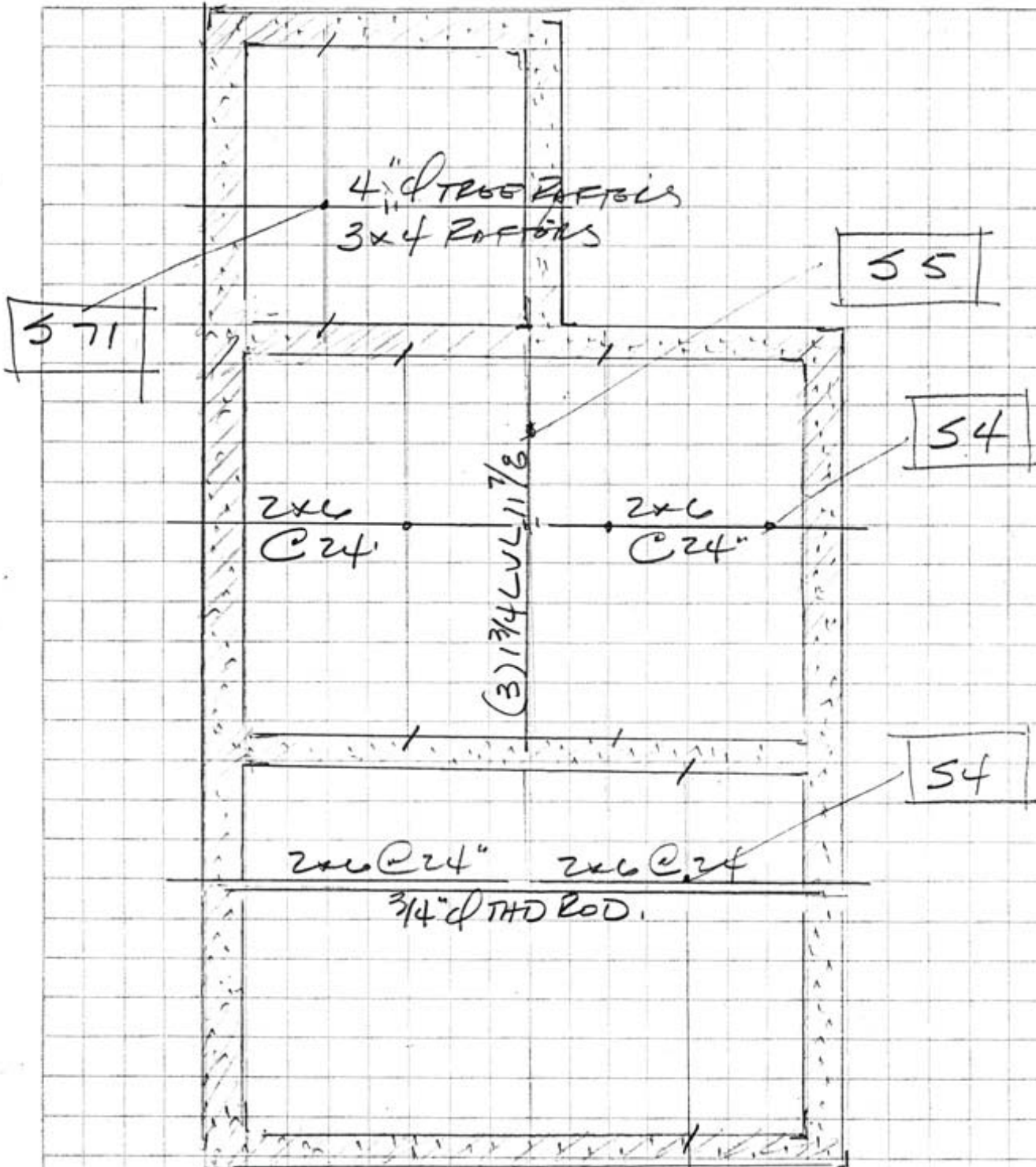
ROOF FRAMING PLAN 1/8" = 1'-0"
